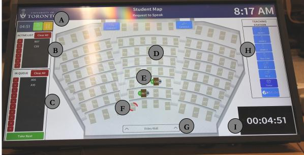
This monitor is mostly used to control the input from student tables, receiving the audio from the microphones either alone or with the video. The only way to use just the video is to mute the student mic.
