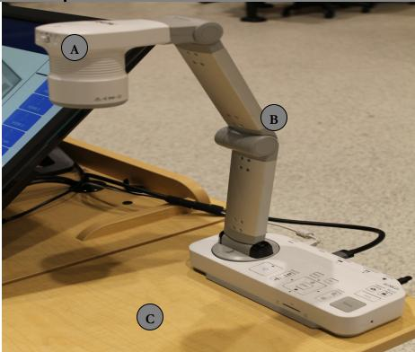
The document camera gives the most low-tech way to display information in the room.; it is the closest relative to the chalkboard. At the simplest, it needs only a pad of paper underneath the camera and a Sharpie for writing. The ideal paper size for the <u>camera</u> is 11"x17". Except that it will not fit on the <u>table</u>. 11"x14" seems to work best, placed in landscape orientation.
