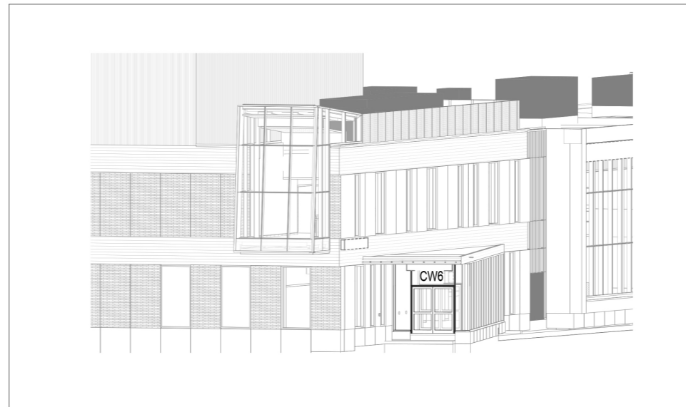
9 3D VIEW OF GLAZING CW6 A353
